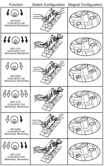
Verify switch cover is oriented correctly for switch configuration. Note that only one, two or four switches can be installed. Three is not recommended.
