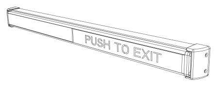
**GENERAL DESCRIPTION:** The 672 Series Request to Exit TouchBar is a non-latching releasing device. It is most often used as a switch to release a magnetic lock. A double pole output is standard, and allows for use when integrating with a monitoring system which requires a signal for legal egress. The device can be ordered to fit 3 standard door openings or can be cut to size in the field. A 24-inch (minimum) pre-connected cable comes standard to make installation easier.
