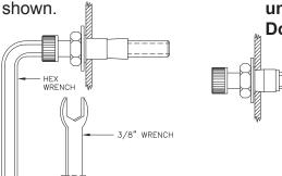
III. Using a 3/8" wrench, rotate the nut clockwise until the nut collapses against the inside of the door skin. Some resistance will be felt. Carefully tighten until nut is secure. Do not overtighten.
