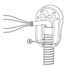
Install door cord onto door and frame. Use all four screws.
