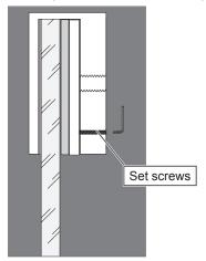
Shim with compression pad to be installed on top of glass opposite the hinge side with the hole for the armature facing toward the "push" side of the opening.
