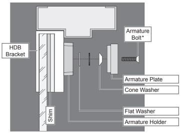
Use bolt supplied in HDB kit. M490 armature must be disassembled to replace armature bolt
