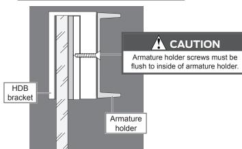
3b Install armature plate.
