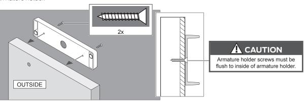
4b Install armature plate as shown for door type (M420/M450 shown).
