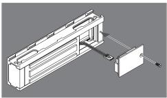
5c Slide magnet onto bracket.
