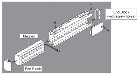
b. Rotate magnet, end blocks and wiring cover as shown, then reassemble.
