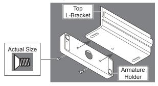
8b Attach armature plate to armature holder.
