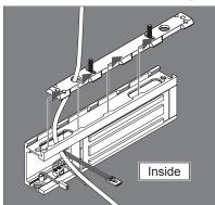
6b DOUBLE LOCK ONLY: Slide second magnet onto bracket. Join block slides into first magnet housing.
