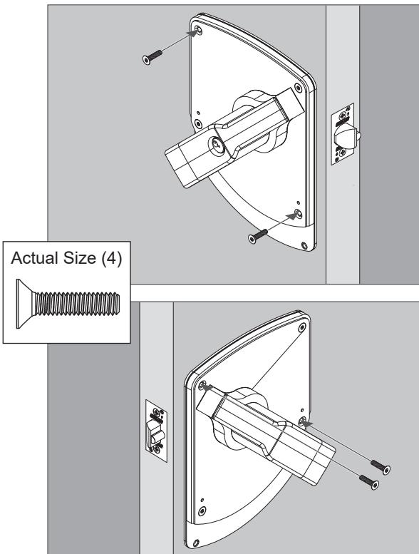
7b Check function. If operation is not smooth, loosen screws, lift trim on door until smooth. Then install surface-mount screws.
