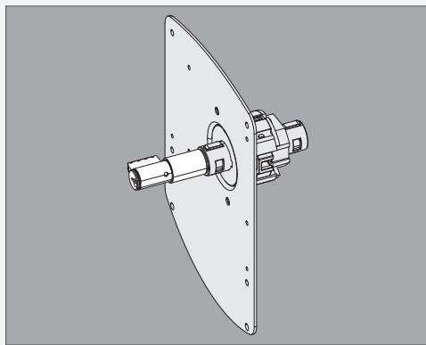
6. Reinstall chassis and subplate onto trim.
