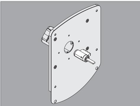
4. From **OUTSIDE**, rotate key cam **CCW** until it stops.
