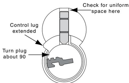
4. There are two shear lines in each chamber; one for the operating keys (change, master, grand master, etc.) and one for the control key. A build-up pin is used to span
