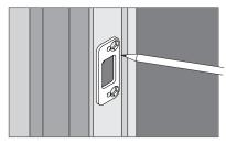
4c If necessary, use chisel, hammer and drill to correct door jamb preparation.
