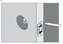
5b Remove bolt and drill two 1/8" pilot holes.
