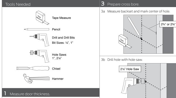
If the door is thinner than 1%" or thicker than 1%", then the lock will not fit properly on the door.
