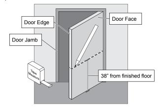
2b Mark top centerline on door face, door edge and door jamb.
