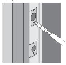
① Mortise for latch strike extends all the way to the edge of the jab to allow for the latch lip.
