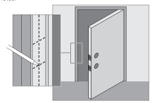
6b For the bolt strike, measure, mark and drill two (2) 1" holes, 11/4" deep, as shown. Chisel out excess material on the sides.
