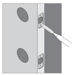
6 Measure, mark and drill holes in door jamb for strikes.
