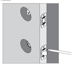
5b Remove latch and bolt. Drill four 1/8" pilot holes.
