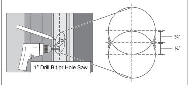
6c For the latch strike, measure, mark and drill two (2) 1" holes, ½" deep, as shown. Chisel out excess material on the sides.
