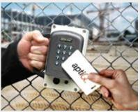
The WPR400 can validate credentials in real time when in range of the PIM400-TD2, which is connected to the access control panel. The WPR400 is capable of operating in cache mode, and when enabled, it keeps a local database of valid access grants. Upon moving the WPR400 to a location that is out of range the local database can be used to verify up to the last valid 1,000 users.
