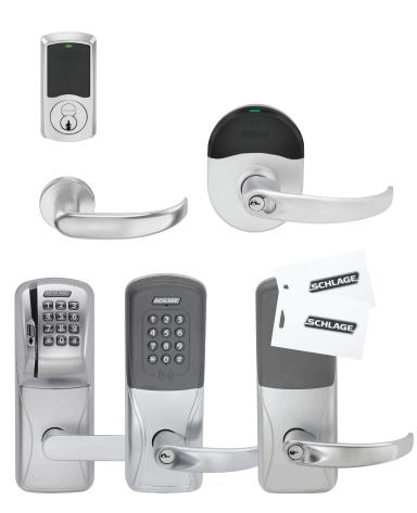
Electronic locks combine the electrified lock, credential reader, door position and request-to-exit switches in one device for simple installation. To accommodate various project requirements, options include standalone and networked wireless or hardwired locks.
