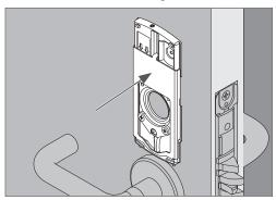
1c Install the alignment cylinder with cylinder spring as shown. Use any slotted screwdriver, lever wrench, or coin to rotate the cylinder.
