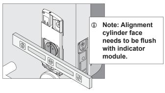
(i) Note: Slot in the alignment cylinder must be vertical after installing the alignment cylinder.
