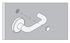
1b Proceed with the appropriate steps to install trim on opposite side. If both trims are installed, proceed to page 15 to complete installation.
