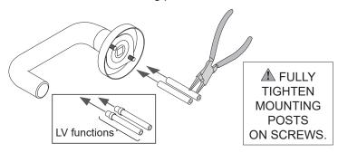
4b Install outside spring cage or spacer.
