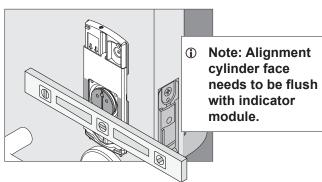
Note: Slot in the alignment cylinder must be vertical after installing the alignment cylinder
