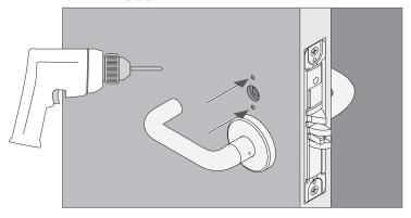
Ib Install the thumb turn.
