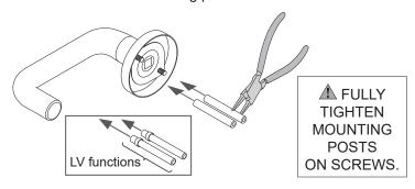
4b Install outside spring cage or spacer.
