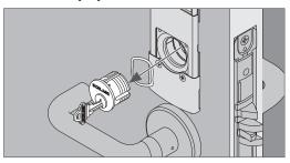
3b Mount the sectional trim. Line up pins on bottom of indicator module with holes on sectional trim, then pivot trim until flush with the door.
