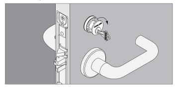
Proceed with the appropriate steps to install trim on opposite side. If both trims are installed, proceed to page 23 to complete installation.
