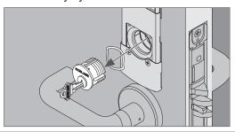
Mount the sectional trim. Line up pins on bottom of indicator module with holes on sectional trim, then pivot trim until flush with the door.
