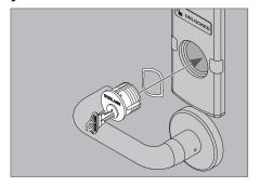
3d Proceed with the appropriate steps to install trim on opposite side. If both trims are installed, proceed to page 23 to complete installation.
