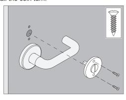
1c Proceed with the appropriate steps to install trim on opposite side. If both trims are installed, proceed to page 15 to complete installation.
