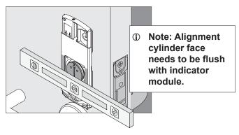
(i) Note: Slot in the alignment cylinder must be vertical after installing the alignment cylinder.
