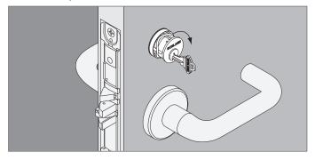
1c Proceed with the appropriate steps to install trim on opposite side. If both trims are installed, proceed to page 7 to complete installation.
