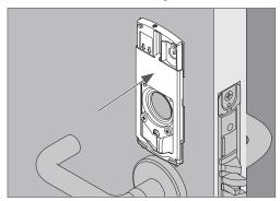
1c Install the alignment cylinder with cylinder spring as shown. Use any slotted screwdriver, lever wrench, or coin to rotate the cylinder.
