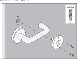
1c Proceed with the appropriate steps to install trim on opposite side. If both trims are installed, proceed to page 7 to complete installation.
