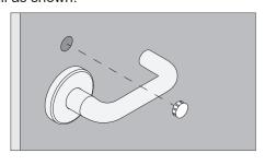
1b Proceed with the appropriate steps to install trim on opposite side. If both trims are installed, proceed to page 23 to complete installation.
