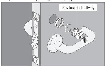
1b Rotate cylinder clockwise.
