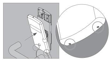
3b Proceed with the appropriate steps to install trim on opposite side. If both trims are installed, proceed to page 23 to complete installation.
