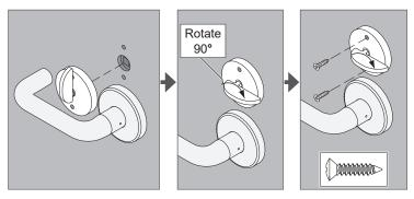
1c Proceed with the appropriate steps to install trim on opposite side. If both trims are installed, proceed to page 23 to complete installation.
