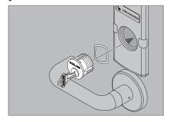
3d Proceed with the appropriate steps to install trim on opposite side. If both trims are installed, proceed to page 15 to complete installation.
