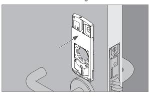
1c Install the alignment cylinder with cylinder spring as shown. Use any slotted screwdriver, lever wrench, or coin to rotate the cylinder.
