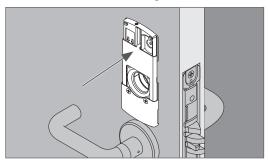
1c Insert key halfway into the cylinder, and install the cylinder with cylinder spring as shown.
