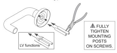
4b Install outside spring cage or spacer.
