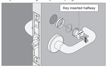
1b Rotate cylinder clockwise.
