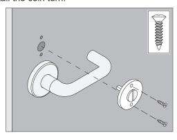
1c Proceed with the appropriate steps to install trim on opposite side. If both trims are installed, proceed to page 23 to complete installation.
