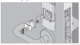
3b Mount the sectional trim. Line up pins on bottom of indicator module with holes on sectional trim, then pivot trim until flush with the door.
