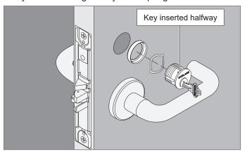
1b Rotate cylinder clockwise.
