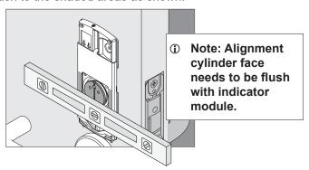
Note: Slot in the alignment cylinder must be vertical after installing the alignment cylinder
