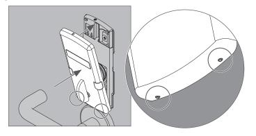
Proceed with the appropriate steps to install trim on opposite side. If both trims are installed, proceed to page 15 to complete installation.
