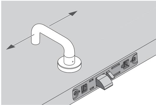
10a Turn a lever inside the mortise lock and ensure both the mortise latch and top & bottom latches retract
