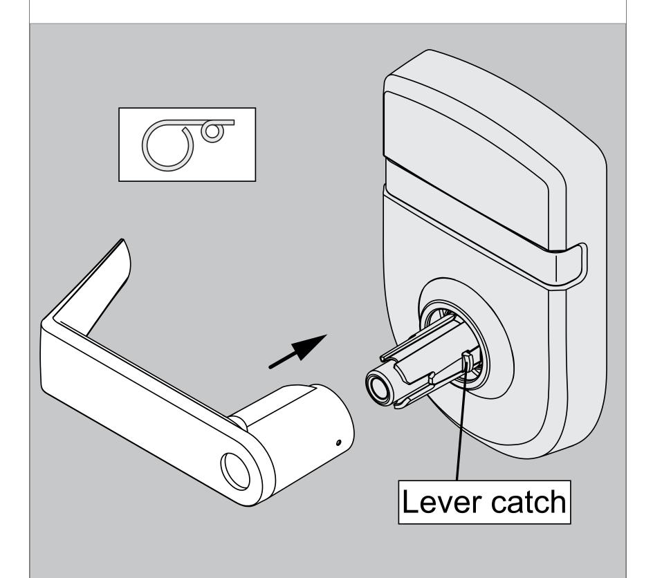
① Note: A pin wrench may be required to depress the lever catch if mechanism is extra tight.
