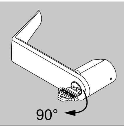
D. With key still at 90° clockwise, rotate key further CLOCKWISE until it stops and then 180° COUNTERCLOCKWISE back to the home position. Remove key from inside the cylinder.
