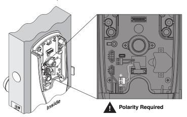
When externally powered, the lock will always fail as-is if power is lost.
